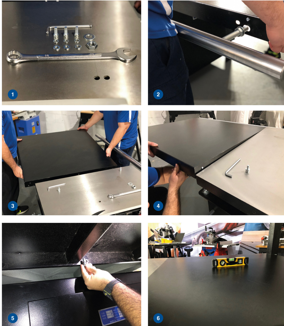
Fig. 1: Use three bolts washers and lock washers to fix the rear table on the main body of the machine.
