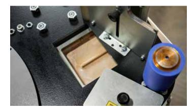
Note that each glue pot comes with a different glue color (White and Transparent). If necessary, add more glue according to the color of the wood and edge tape to be used. do not mix the glue colors.
