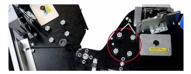
• If the top of the shaft is angled towards the back of the machine, loosen the 5mm Allen bolts at points A (see figures below) and tighten (about 1/4 turn) the hex screws also at point A. Check the square again. If corrected, retighten the Allen bolts.
