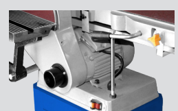
Dust collector port
