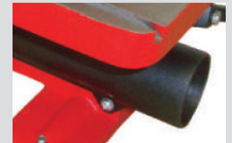
Dust collector port
