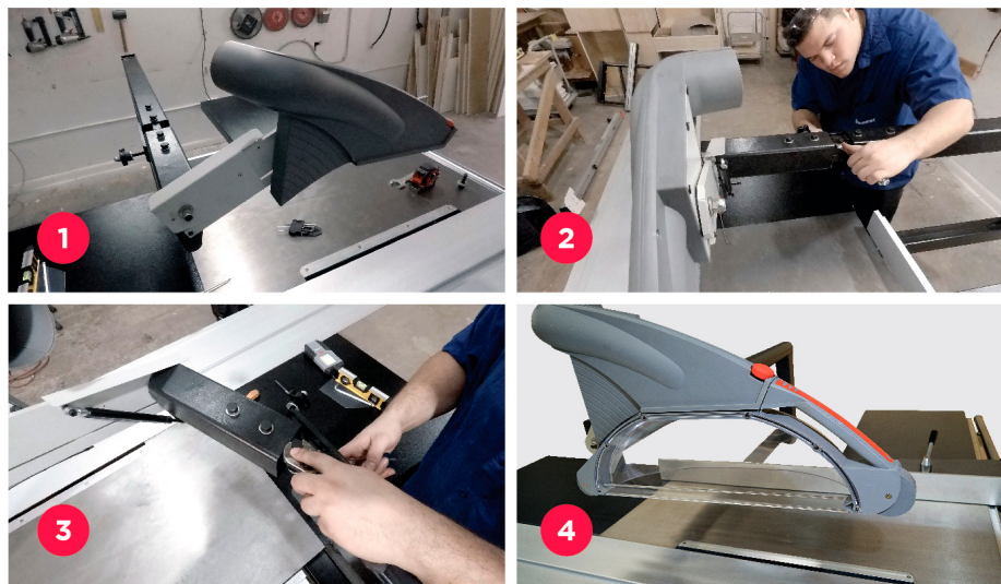
Fig. 1: Attach the saw guard to the frame.
