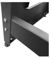
3. Place the adjustable hexagonal feet and put the machine on the floor. Set the positioning of the feet until the machine is level, then tighten the nuts next to the plate, as shown below:
