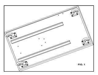
2. TO ASSEMBLY, FIRST PLACE THE BASE PLATE UPSIDE DOWN AND ATTACH THE FOUR CASTERS TO THE HOLES PROVIDED AND TOGHTEN WITH THE WRENCH. FIG.1
