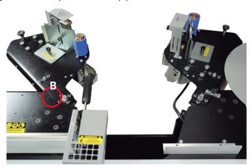
• Move the other glue pot into place, coupling it to the equipment, as shown below:
