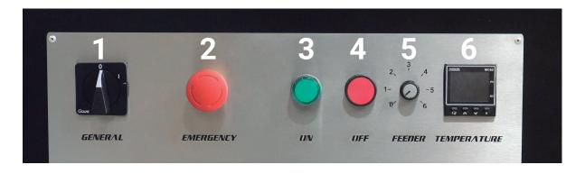
1. Main on/off Switch: This switch powers the control panel, but does not turn on the machine.
