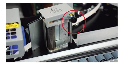
If you want to decrease the thickness of glue, slightly turn glue knob (B) counterclockwise. If you want to increase the thickness of glue, turn glue knob (B) clockwise. Note that small changes (about 1/4 of a turn) already cause a considerable change in glue thickness. Find the ideal amount, which can vary depending on the type and material, glue and the temperature being used.
