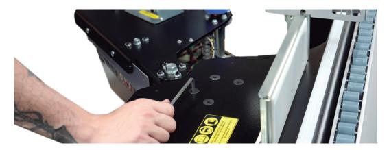
5. Open the extension tables according to your need, making sure to fit the latches into the side holes as shown in the picture:
