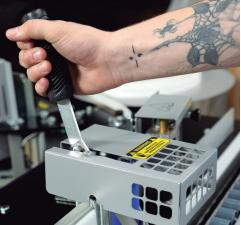
CAUTION: Risk of crushing and cutting. Do not bring your hands closer than 10 cm / 4 inches from the tape knife. Do not wear gloves or loose clothing when operating this equipment.
