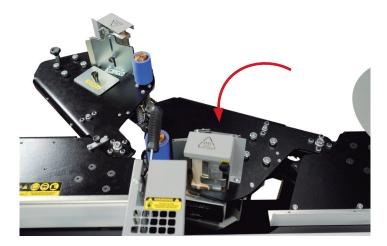
• Attach the glue pot assembly again to the machine body and tighten the knob (C) as shown below
