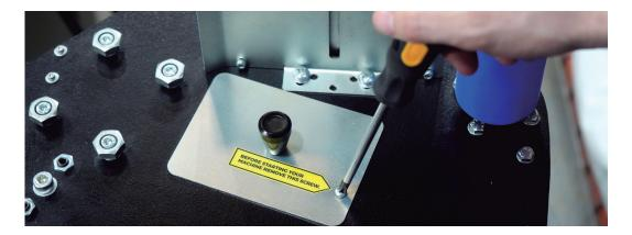
9. Use locking bracket to prevent the Glue Pot to move, as shown below.
