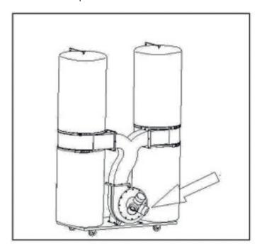
The dust collector is now ready to be placed into service. Before connecting to a power source, be sure the power source is properly grounded and is of proper voltage and amperage.
