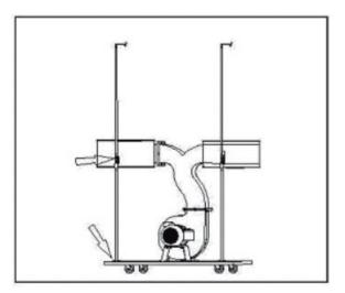
Next, hang the two bags (H) from the support rods. Then attach the two filter bags and two collection bags to the collectors using bag clamp.
