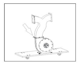
4. Next install the two collectors (C) two packing (I) to the outlet as shown in Fig5.
