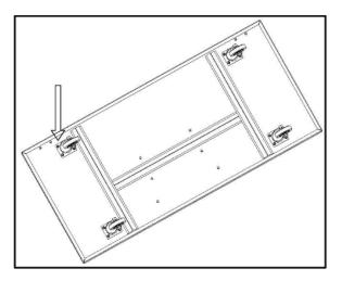
2. With the motor base, collector body & fan/motor assembly in place, secure it to the base plate using the screw and washers provided as shown in Fig 2.
