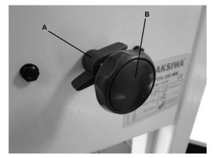
To adjust the lower hand wheel, loosen the nuts (A) located at the rear of the machine and tighten or loosen the screws (B) in order to find the alignment of this handwheel. After correcting the problem, secure the nuts (A) again to lock. Check the figure below.
