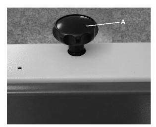
15 Install the special Slotted screw and washer (A) on the left side of the machine, so that it serves support for the push stick (B) that comes with this equipment. This stick is indispensable for the cutting small parts. Look the following picture.
